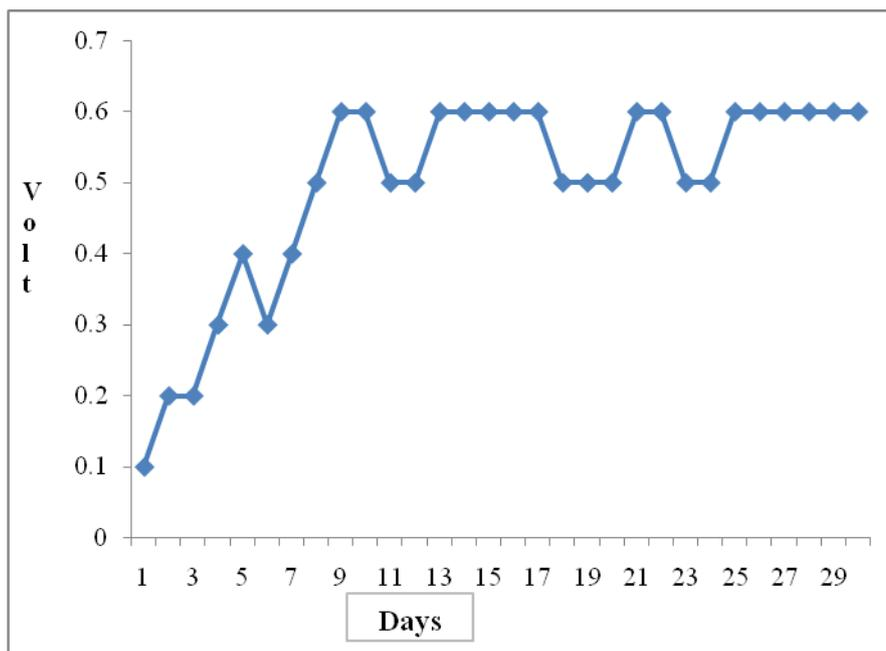
**Figure 5: Voltage generation in single chambered P-MFC using Chlorophytum plant**
