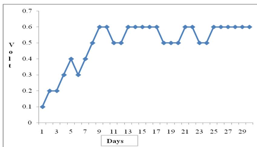
Figure 6: Effect of copper on voltage generation in a double chambered P-MFC
