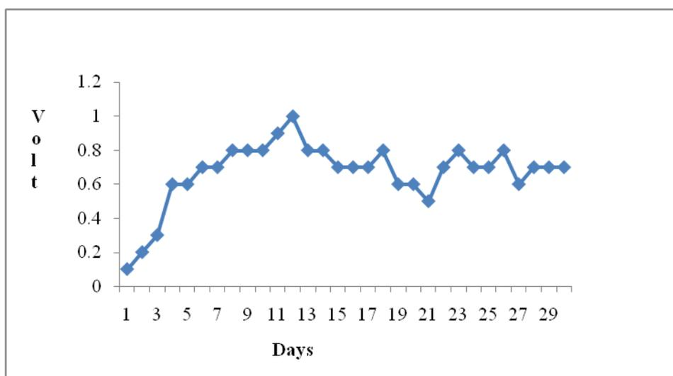
**Figure 4: Voltage generation of double chambered P-MFC using Chlorophytum plant**
