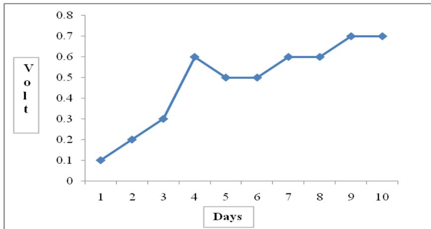
Figure 7: Effect of carbon on voltage generation in a double chambered P-MFC
