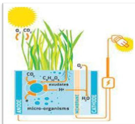
**Figure 1: Schematic Representation of P-MFC in power generation [6].**
